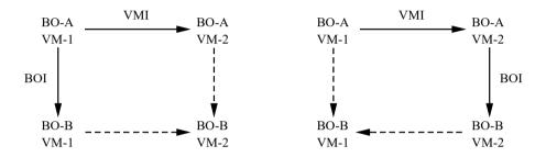
Similarly, one VMI programme, run on either the original Base Oil/Performance Additive Package or the interchange Base Oil/Performance Additive Package System, will cover both systems.
